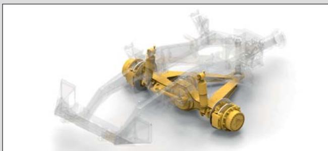
For comfortable productivity, front-suspension damping helps minimise vibration, while a superior suspension seat reduces the roll often experienced in off-road conditions.
